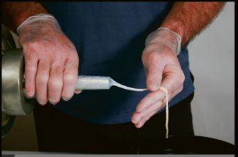
Slide casing onto stuffer tube using forefinger and thumb until full length is loaded onto tube.
