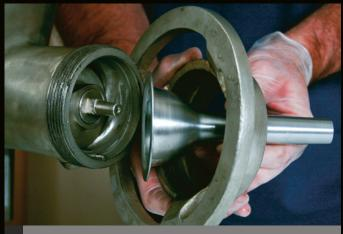
Remove grinder knife & plate before mounting stuffer tube to grinder.
